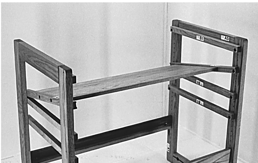
Lift up front of the Monitor Shelf Assembly, and attach it to the Front Legs as shown. Use screws and washers from the D2 hardware bag. Snug screws up but do not tighten yet.
